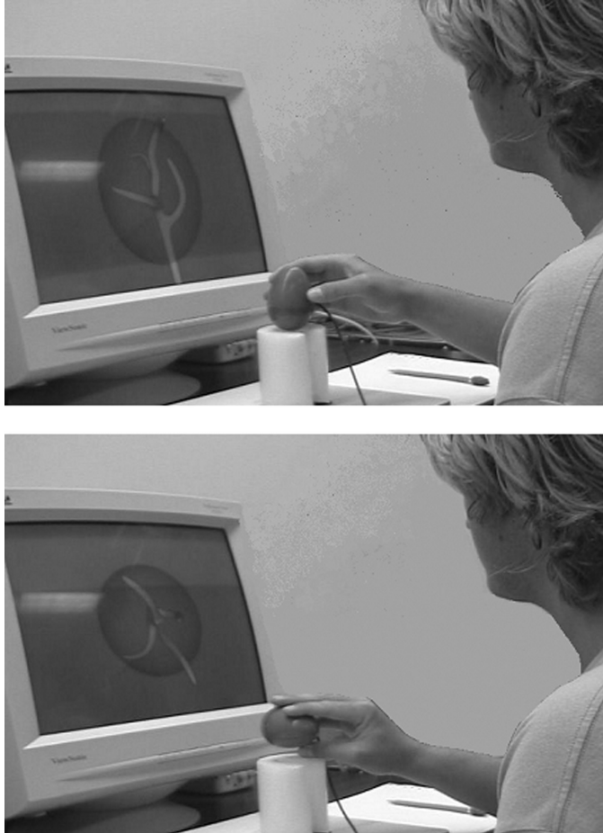
Fig. 4. Experimental set-up in the interactive conditions of Experiments 2 and 3. Note: The egg-shaped control device contained a 3 df motion tracker, so that rotations made with this device were replicated by the on-screen object in real time.
